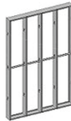
NON-LOAD BEARING WALLS
